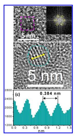
Figure 2. (a) HRTEM image of a typical N-GQD. Inset: fast Fourier transform image of a selected area (pink square), the hexagonal honeycomb structure, is indicated. (b) HRTEM image and the (c) line profile of the selected N-GQD. The layered structure with an interlayer spacing of 0.384 nm is observed. The sample was prepared by microwave heating for 5 min.
