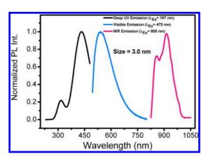
Figure 4. Normalized PL spectra of the N-GQDs ( $\Phi$  = 3.0 nm) excited by various wavelengths.
