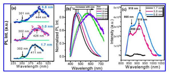
Figure 5. PL spectra of the N-GQDs with different sizes. (a) Deep UV PL spectra of the N-GQDs excited by 197 nm laser measured at 300 K. (b) Size-dependent visible PL spectra of N-GQDs excited by 375 nm laser. (c) NIR PL spectra of the N-GQDs excited by 808 nm laser.
